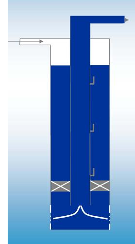
In response to gas pressure the liquid in the casing is forced into the tubing
