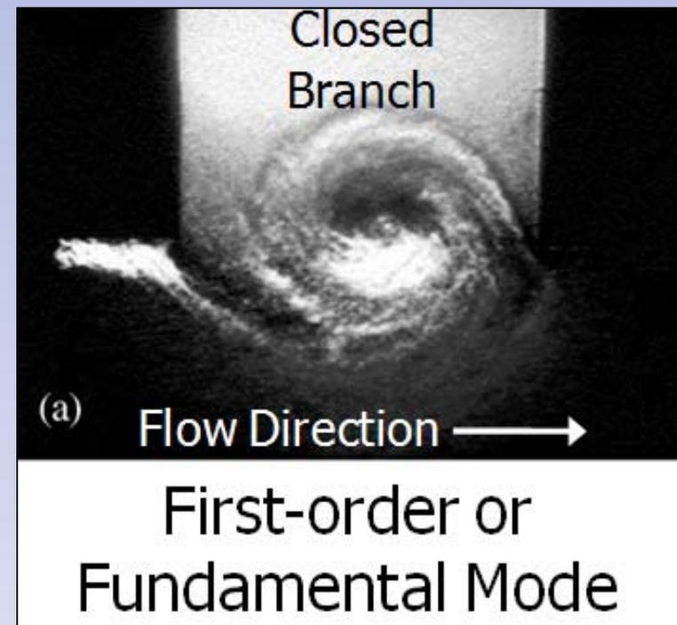
Side-branch Pulsation in Water (S. Dequand, et al.)
