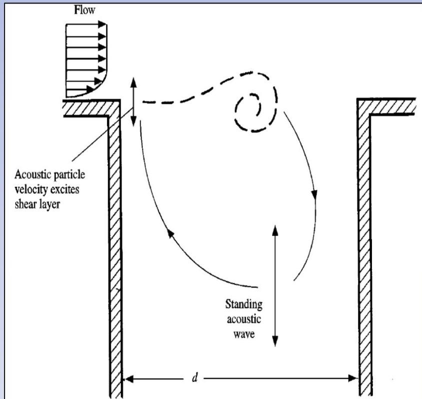
Feedback mechanism of flow-excited acoustic resonances at closed side-branches (Ziada & Shine, 1999)
